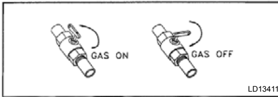
Figure 1 - Typical Furnace External Manual Gas Valve
