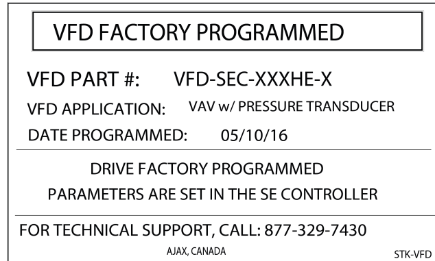
Figure 1: Label on unit/VFD for VAV with pressure transducer
