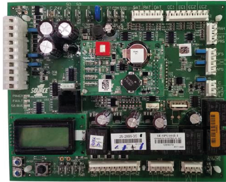
Figure 41: Communication board installed
